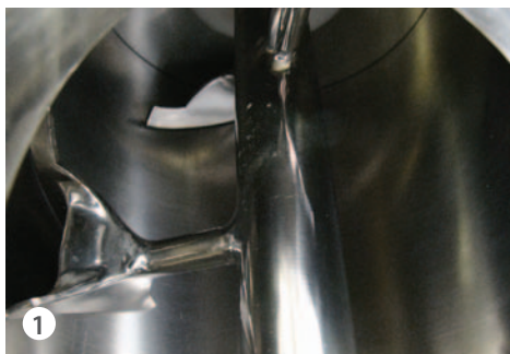
Internal chamber with welded ploughs, and polishing treatment
