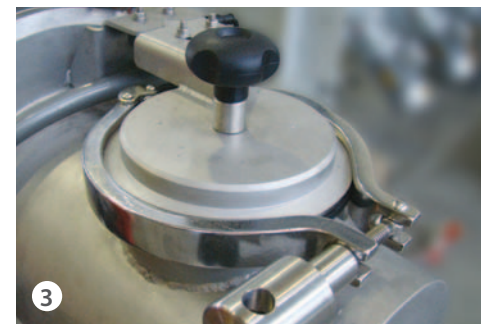
Closure plug for the feeding door
