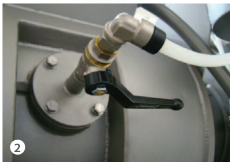
2 Mixing chamber, endplates excluded, equipped with heat exchanger (as an option)
