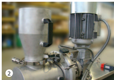
Funnel for product feeding/unloading
