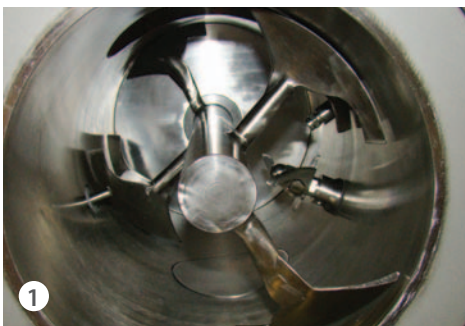
1 Internal chamber with welded ploughs, and polishing treatment
