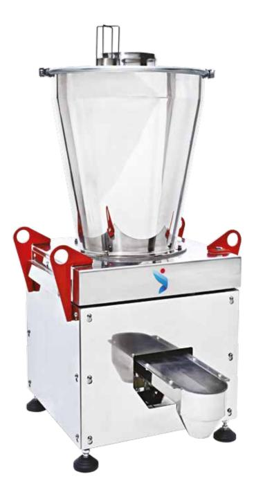
The C Series vibrating channel feeders, thanks to their operating principle, feed every product without damaging it mechanically or affecting its exterior. This distinctive feature makes them suitable for feeding fragile raw materials with irregular sizes such as tablets, granules, fakes and stringy products. Available in both volumetric and loss-in-weight releases with electronic twin load cell system, they ensure accuracy and reliability.
