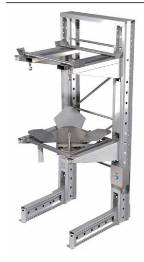
The EBQ station is the ideal device for unloading BIC-BAGs. An efficient cloverleaf shaking system operated by electro pneumatic pistons ensures a high level of operating comfort even with materials that are difficult to extract. Thanks to a complete range of accessories we are able to configure the big-bag emptying station to the specific demands of the customer.
