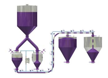
Full pipeline continuous is suitable for **long distances**: the use of two vessels with smaller dimensions and overall dimensions than the same cycle carried out with a single tank, allows optimal performance.
