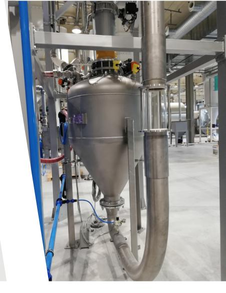
Pressure vessels for dense phase pneumatic conveying of bulk materials
